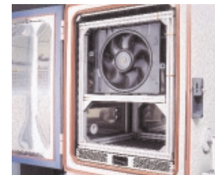
Climatic chamber made by Weiss-Klimatechnik (Schunk Group). Regulation of humidity between 10%–95% is possible, the temperature can be adjusted from -40 °C to +180 °C
