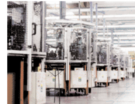
production hall with modular automatic rotary tables
